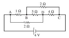
Calculate the current drawn from the battery by the network of resistors shown in the figure.
